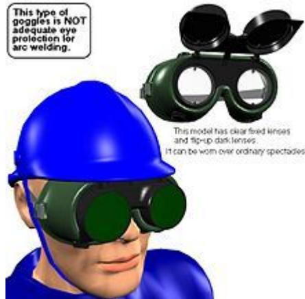
Gas welding/cutting goggles and safety helmet
