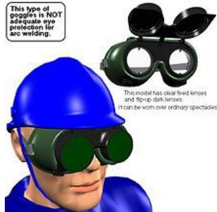
Gas welding/cutting goggles and safety helmet
