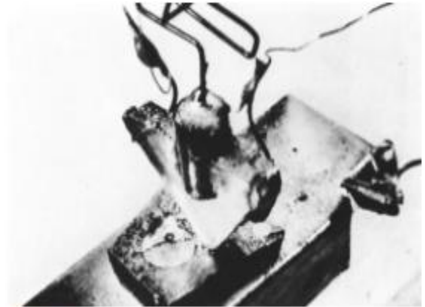
Figure 3.1 The first transistor. (Courtesy Bell Telephone Laboratories.)
