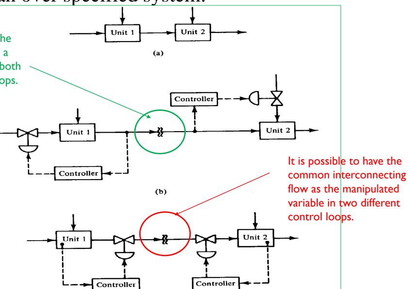
Generate the control loop configuration for a simple chemical process
